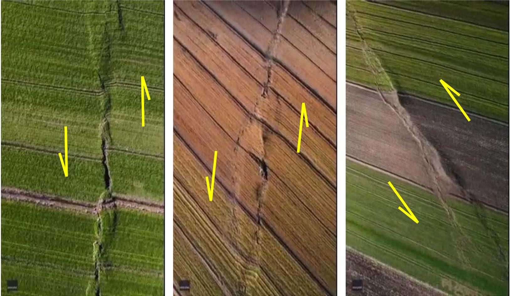
Surface ruptures observed in the Kahramanmaraş located in the northern part of the earthquake-affected area. The ruptures have affected farmland and displaced irrigation channels and roads.
