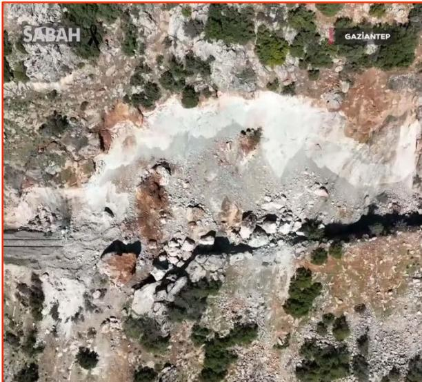
Rockfalls were triggered along slopes in Islahiye area, causing damage to the railroad. Landslide prevention measures were taken, however the nets failed due to the large volume of the mobilized material.
