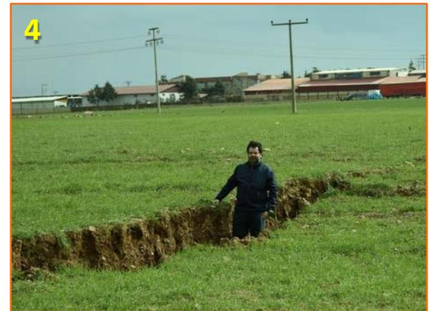
Surface ruptures caused damage in roads, pavements and warehouse perimeter walls and deformation in fields and concrete slabs. **1:** Surface ruptures in a field. **2:** Cracked and disrupted perimeter wall. **3:** Deformed concrete slabs. **4:** Large gaps were formed along the observed surface ruptures.
