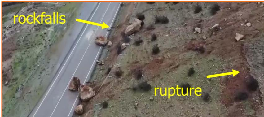
Surface ruptures in Kahramanmaraş. They affected roads and farmlands and triggered rockfalls and landslides along their path. The mobilized material reached adjacent segments of the road network resulting in temporary traffic disruption in lanes.
