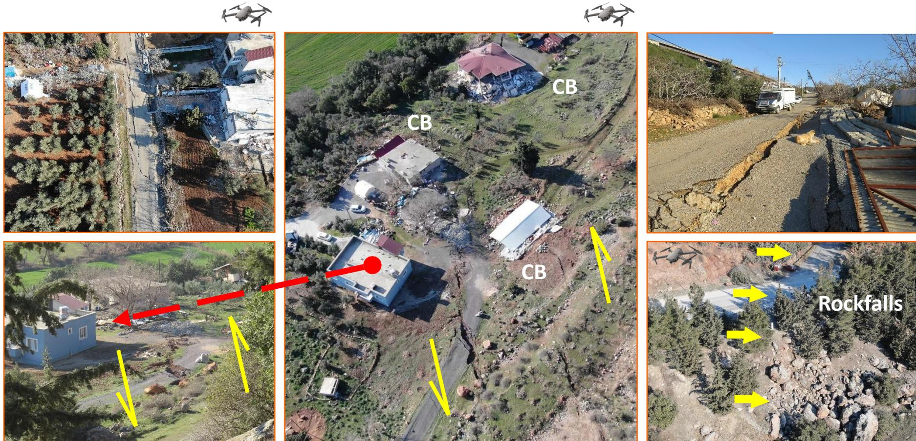
Buildings and infrastructure located within the deformation zone of the coseismic surface ruptures suffered very heavy structural damage including total collapse. The buildings in this site were totally destroyed (CB: Collapsed buildings in the middle figure). Along the same ruptured zone, rockfalls were also triggered.
