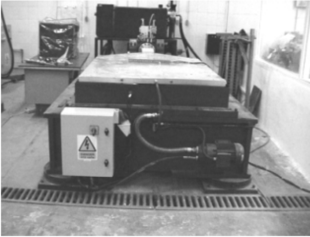
Figure 9. The IIEES shake table test facilities.
