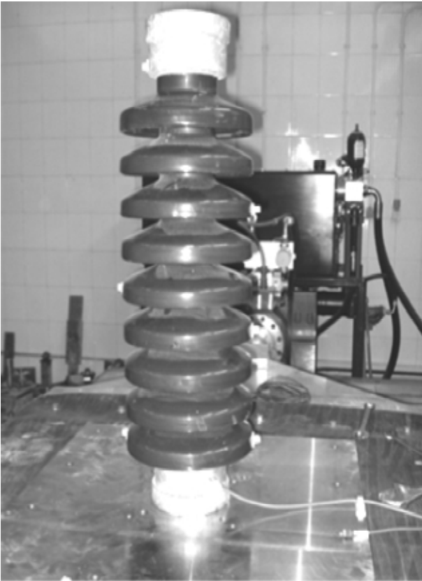
Figure 3. 63kV Post Insulator specimen.
