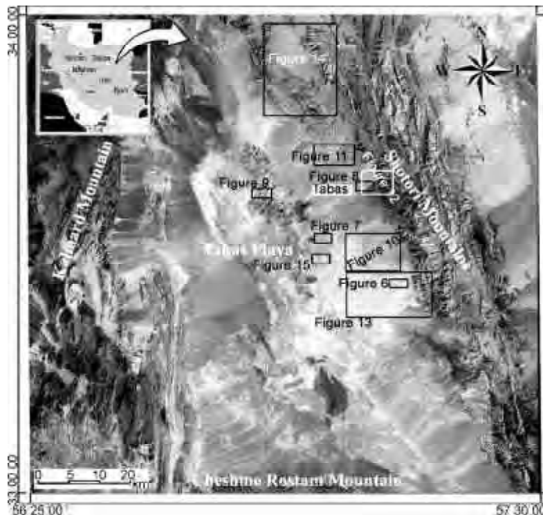
Figure 1. Landsat ETM+ Image of Tabas area, processed by Erdas 8.5 Software Package after combination bands No: 1, 2&3 assigned to RGB. The city of Tabas is located between the Shotori mountain to the east and the Tabas playa to the west.
