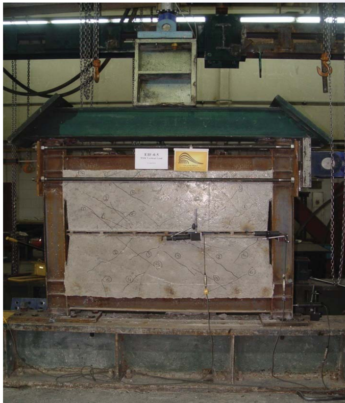
Loading the specimen in vertical direction
