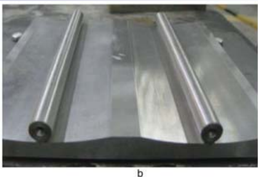
The prototype sample of the OPRCB isolator. (a) The set of the prototype OPRCB. (b) One pair of rolling rods on their concave beds
