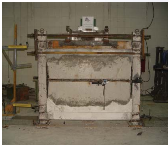
Repaired specimen (with Grout)
