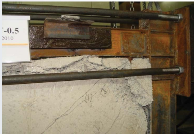
Corner crushing at corner of an engineered infill panel, with top gap
