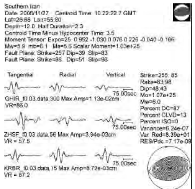
Figure 4. The result of data inversion from GHIR (distance of 320km) and ZHSF (distance of 560km) stations for the main shock of Qeshm earthquakes with waveform fit (bottom of the figure) as compared with Harvard University results (top of the figure). The data are shown as solid lines and the synthetics are dashed.
