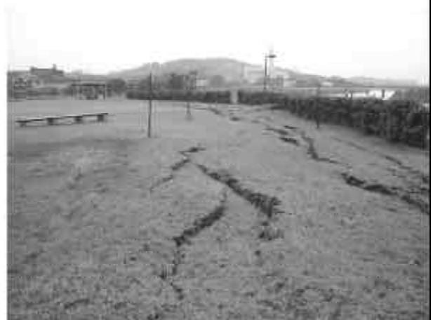
Figure 13. Large ground fissures due to liquefaction at the Sabaishigawa Kaishu-Kinen Park in Makhara-Kashiwazaki. The park was constructed on a sandbar along the Sabaishi river.
