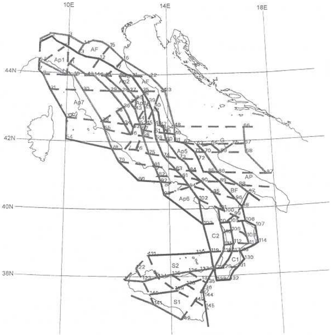
Figure 1. Morphostructural map of the study area. Violet lines are the lineaments of the first rank, blue lines are the lineaments of the second rank, green lines are the lineaments of the third rank, continuous lines are the longitudinal lineaments, discontinuous ones are the transverse lineaments. Nodes are numbered from 1 to 146. Ap, Apennines; AF, Adriatic foredeep; AP, Apulian platform; BF, Bradanic foredeep; C, Calabria; G, Gargano Promontory; S, Sicily.
